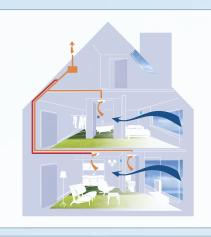
The diagram illustrates a typical "System 3" central extract duct layout, focusing on the 'Best Practice' that the toilet extract is separate to, or positioned in line between the kitchen extract and the extract unit. The unit should only be positioned in the loft, if it is positioned within the heated envelope of the building.
